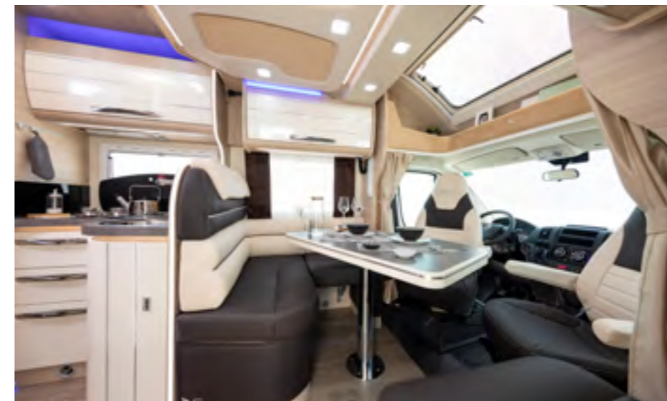
Cab seats can be rotated 180° with covers coordinated with the upholstery. Double-density expanded polyurethane seats.
