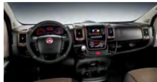
Steering wheel with typical inclination of a car and possibility to be adjusted axially with a travel of 50 mm.
