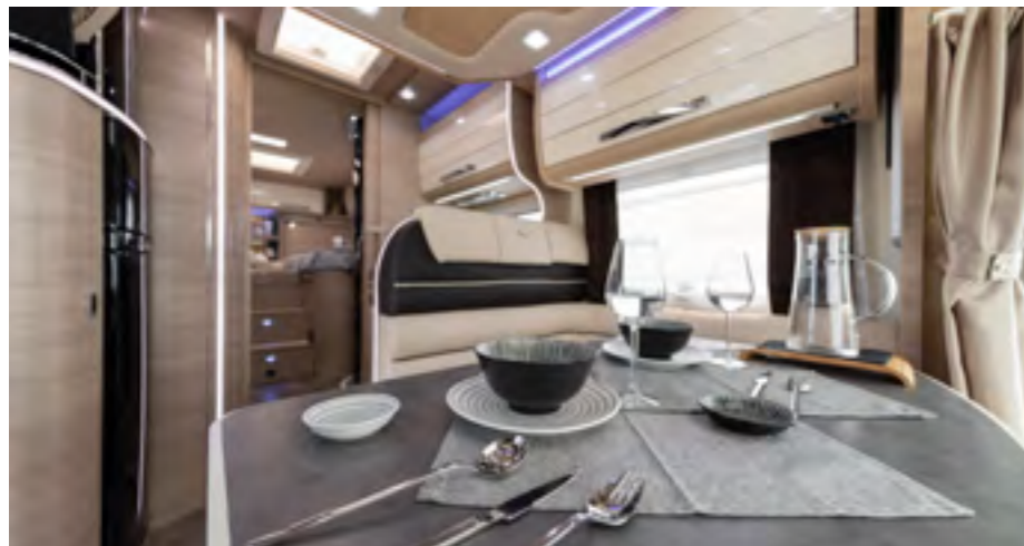
Island dinette table with 360° rotation to find the best position according to the needs of travelling or parking.
