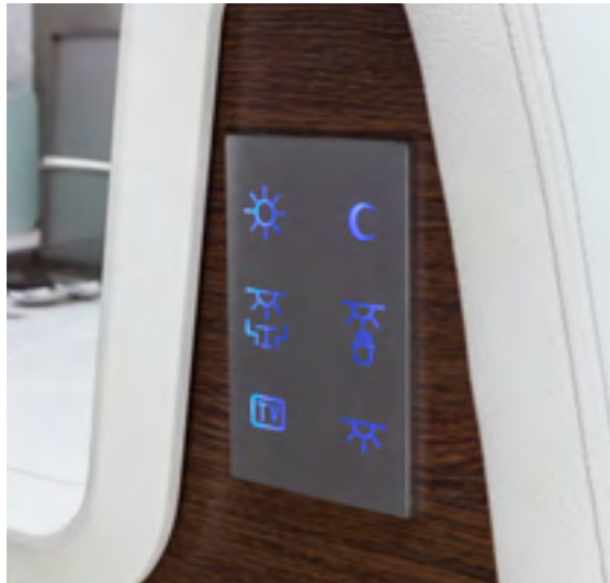
Lin Bus smart technology that allows the adjustment of the lights of the rooms with proximity sensor.
